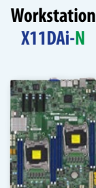
Workstation X11DAi-N 2 Ports NVMe 16 DIMMs, 2x GbE, 4 PCI-E 3.0 x16, 2 PCI-E 3.0 x8 1 M.2, 7.1 HD Audio
